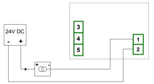
Figure 4.4. Connection of 2-wire current converters
