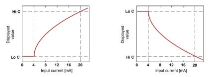
Figure. 9.3 Normal ("Lo C" < "Hi C") and inverted ("Lo C" > "Hi C") characteristic
