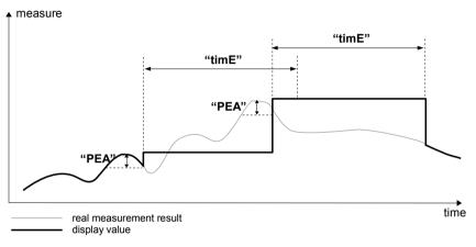
Figure 6.2. Process of peaks detection
