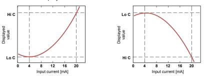
Figure. 9.2 Normal ("Lo C" < "Hi C") and inverted ("Lo C" > "Hi C") characteristic
