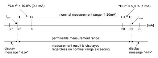
Figure 7.1 Example of definition of permissible range of input signal -"Lo r" and "Hi r" parameters
