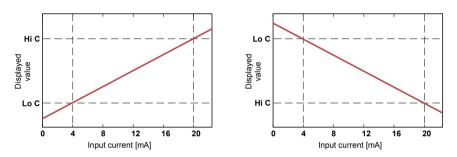
Figure. 9.1 Normal ("Lo C" < "Hi C") and inverted ("Lo C" > "Hi C") characteristic
