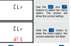
Hold the  $\fbox$  button to confirm the setting and press  $\swarrow$  to return to the main set up menu.
