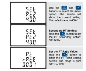
The PT Rate is the PT Primary divided by the PT Secondary. For Example: Voltage Transformer - 11000÷110=100, so the PT Rate would be 0100 and the PT2 would be 110.
