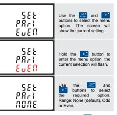
On completion of the entry procedure, hold the E button for 3 seconds until the selection stops flashing.
