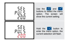
Use the price and P buttons to choose the desired pulse rate. To save the new setting, hold the E button for 3 seconds until the selection stops flashing.
