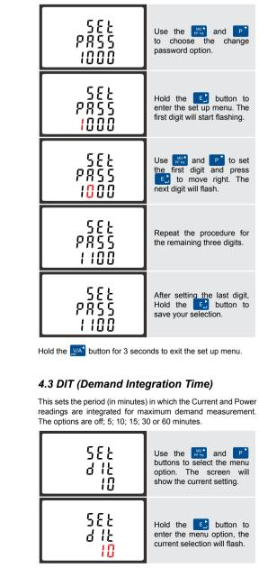
588 Use the buttons to select the d 12 required option. 20 588 Hold the 📑 button to d 12 confirm the selection 20
