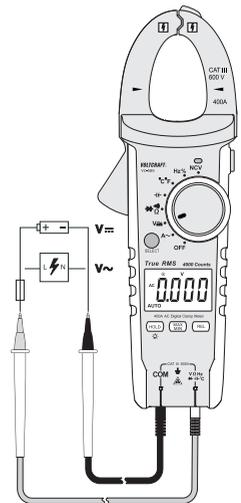
**Proceed as follows to measure direct voltages "DC" (V  $\overline{\text{---}}$ ):**
