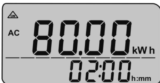
**Note** For kWh in DC power system long,press (>2 Secs) yellow
