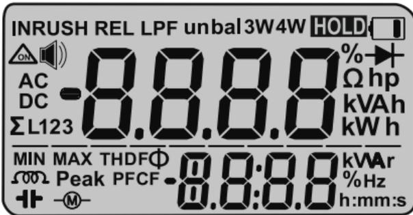
LCD of Clamp meter is as shown above. The digital display shows measured value with sign. Description of remaining symbol is as follow
