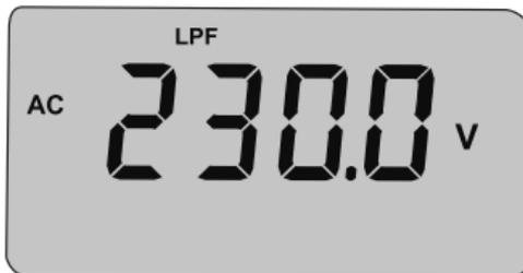
Fig 8.2 Low Pass Filter mode
