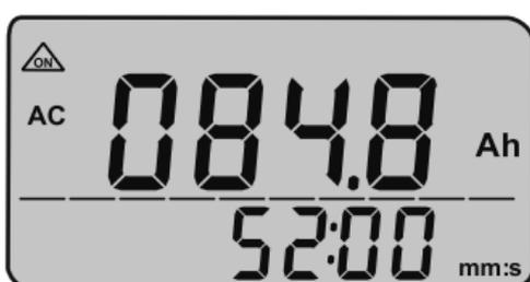
**Note** For Ahr in DC current, long press (>2 Secs) yellow function key clamp meter enters In DC current mode. Now Press **REL** and **INRUSH** key simultaneously, clamp meter will start measuring DC Ampere hours.
