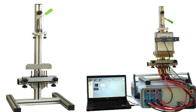
ER10H.3 single position rack with quick connector
