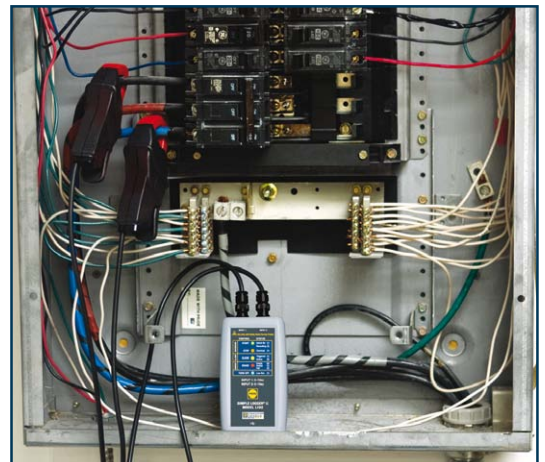
L102 recording two phases of primary feed.
