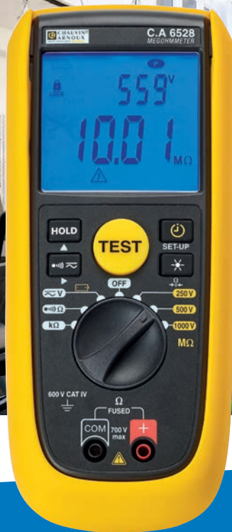
CA 6528 digital insulation tester
